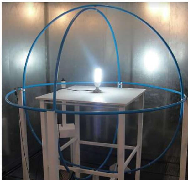
Figura 4 – Antena Loop.
