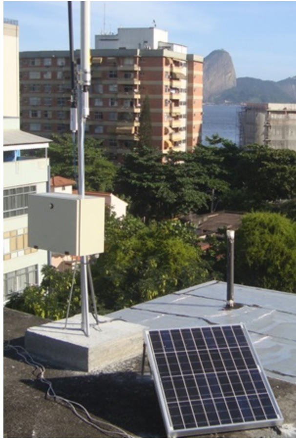
Figure 3.5: ReMoTe's testbed node - External Mesh Network node.
