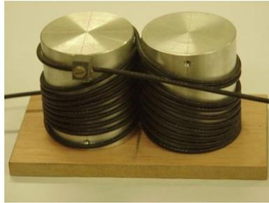
Figure 2 – Photography of the JIS6863 mode-scrambler where 3.4m POF length is wrapped in figure-of-eight around two metallic cylinders.
