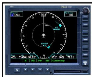
Figura 3.5 - Cockpit Display of Traffic Information – CDTI.
